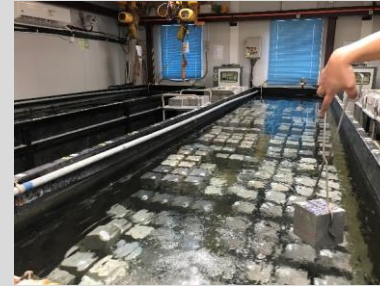
Manually placing test samples into curing tank
