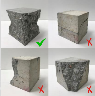
Identification of fracture pattern
